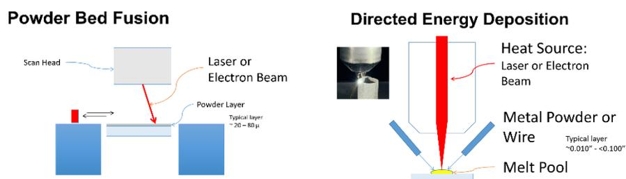
**Picture 3:** Principle Differences between powder bed fusion and deposition method [1]
