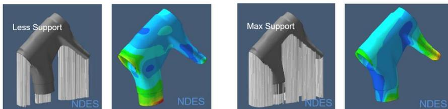
**Picture 12:** Study of varying support structures
