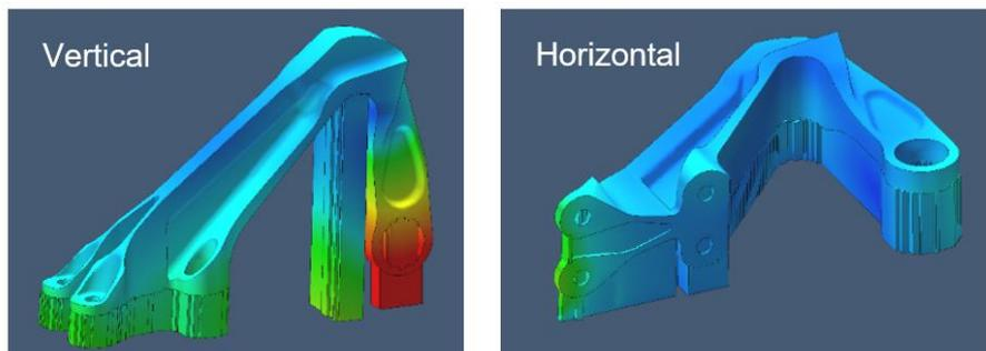
**Picture 11:** Different build orientations result in distinct part distortion
