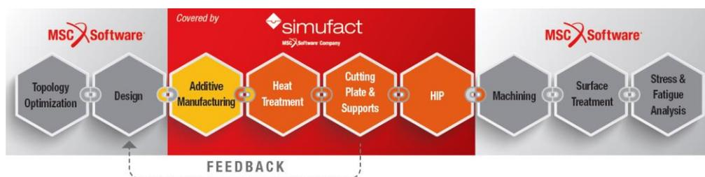
**Picture 8:** Process chain at AM processes
