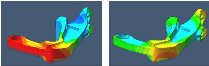
**Picture 10:** Effect of different strategies to remove the base plate and support structure
