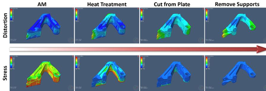
**Picture 13:** Simulation of an entire process chain
