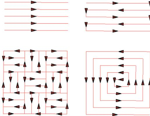
**Picture 4:** Several scan pattern – unidirectional (upper left), bidirectional (upper right), checker board hatch pattern (lower left), spiral hatch pattern (lower right)
