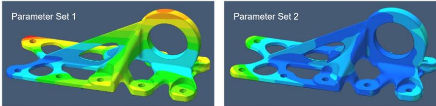
**Picture 9:** Influence of process parameters on final part distortion
